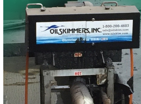
Guard rail mounted Model 6V oil skimmers were installed to remove heavy oil from scale pits at a steel mill. System features a steam heated Hi-Flow Oil Discharge Package to maximize the flow of recovered oil to the centralized collection vessel.
